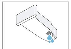
Make sure that you insert the condensation container before operating the appliance.
